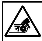
**Caution! Pinch point entanglement.** Pinch point hazard exists in area indicated. Shut down the machine before performing maintenance, repair, or adjustment.
