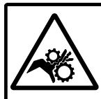
**Caution! Moving parts.** Moving parts can crush fingers or hand. Keep hands and fingers away from moving parts in area indicated to avoid injury.
