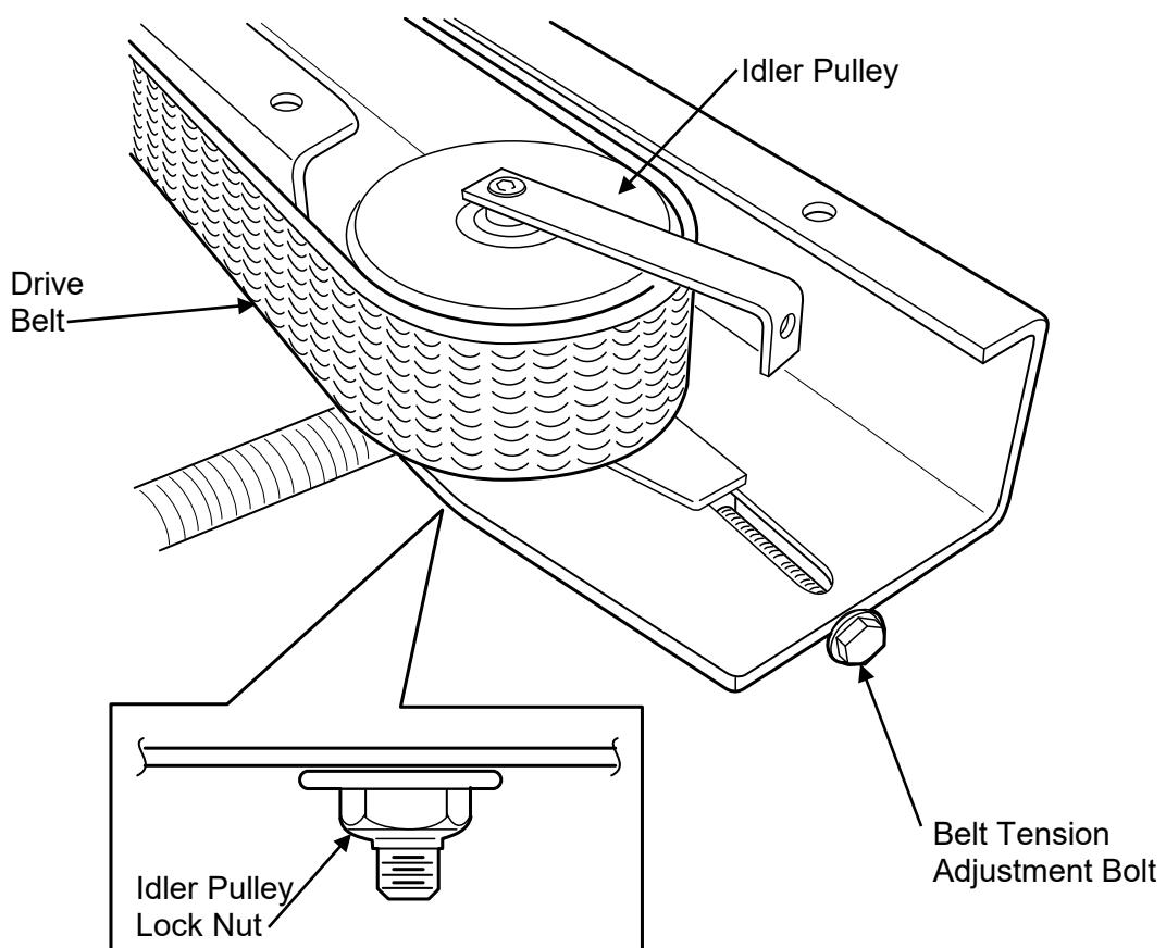
Use the belt tension adjustment bolt to loosen the drive belt enough to remove it from the drive and idler pulleys.
