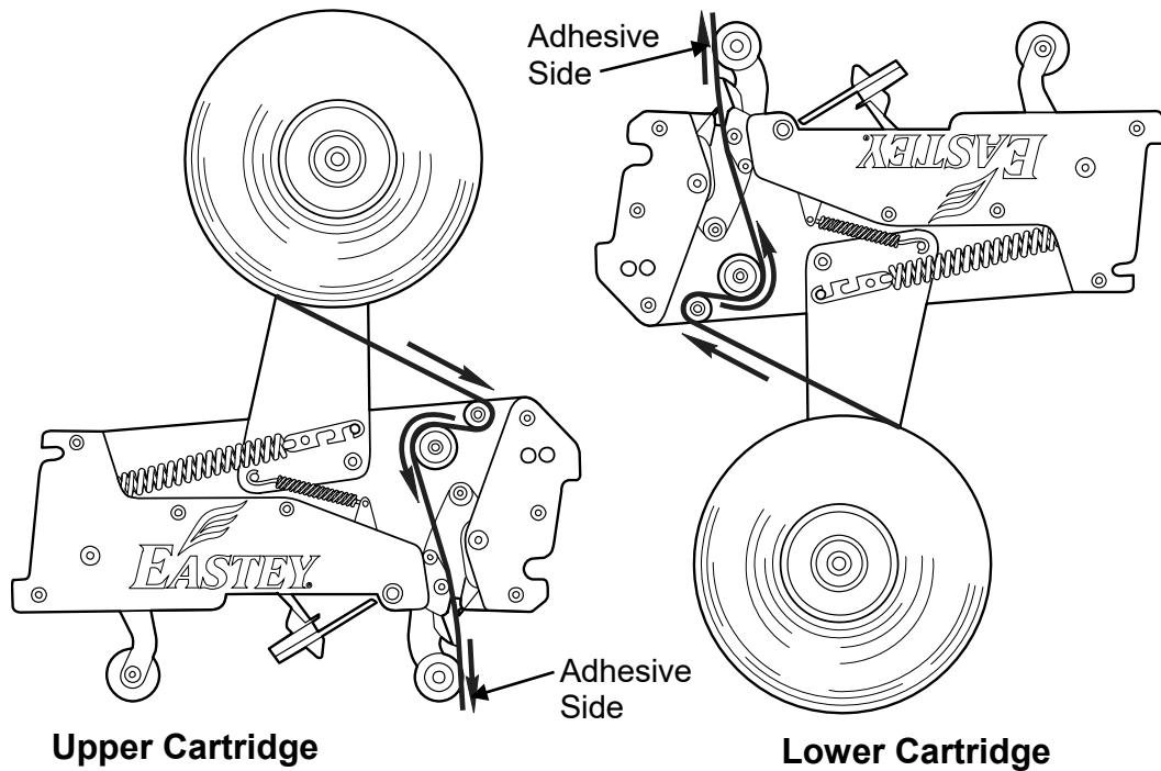
**Reinstall the Lower Tape Cartridge**
