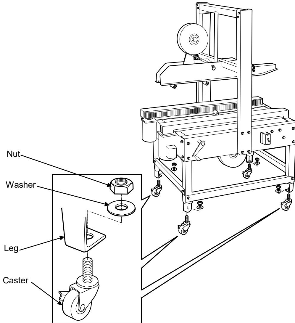
**CAUTION!** When raising the case taper off the floor to install the casters, use proper equipment to lift the case taper. Ensure the SB-2 HD Case Taper is secure and will not shift while the casters are being installed.
