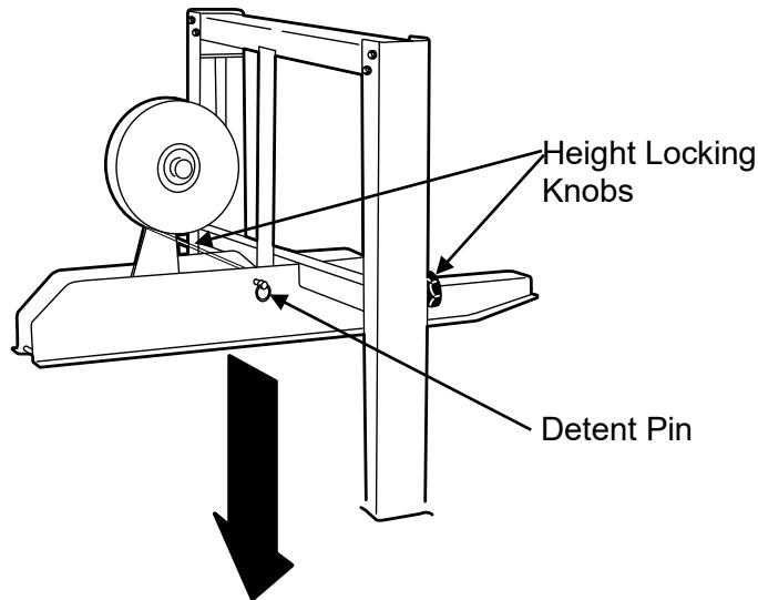
Lift the upper cartridge up and out of the machine.
