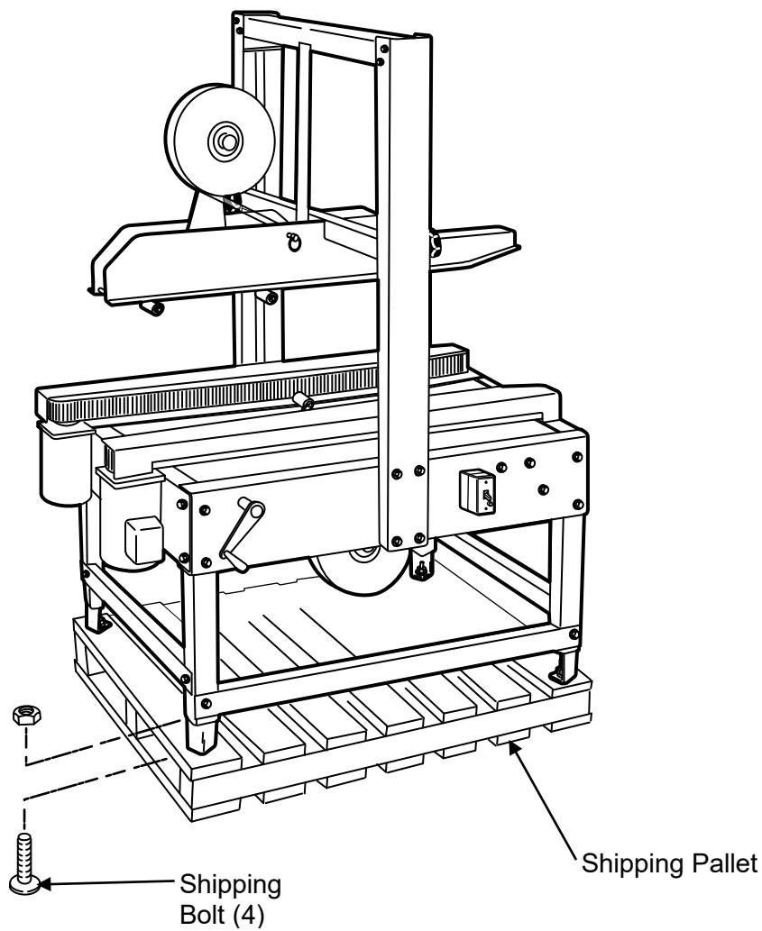
Lift the SB-2 HD Case Taping System from the pallet.
