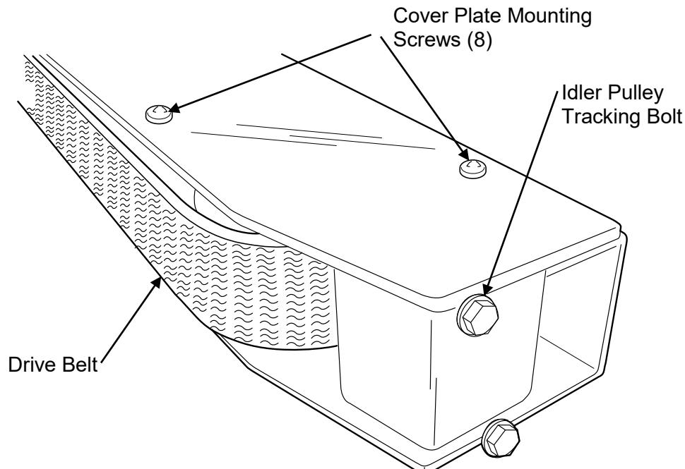
Loosen the idler pulley locking nut located under the idler pulley
