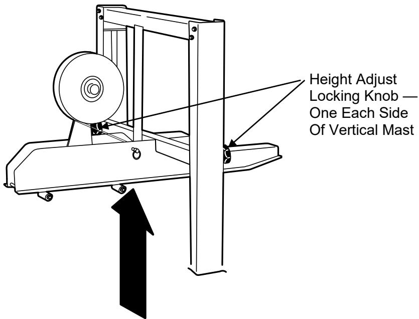
After raising the top taping head up, remove the lower taping cartridge from the bottom section by holding both lift points and lifting leading with the rear lift point first, raising the tape cartridge upward, out of the lower tape head seat.
