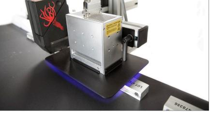
2) Standard bracketry allows Squid UV LED to mount directly to your existing manufacturing line.
